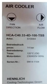
In combined coolers, the individual data for several coolants is provided separately on the marking plate!
